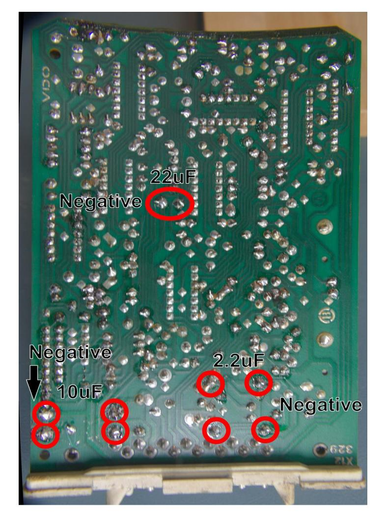
After you have soldered in new capacitors you will need to "reflow" the solder joints on the rest of the board.
